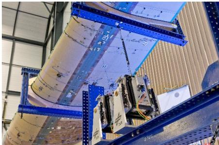
Full body modal analysis in aircraft engineering to manage vibrations of the wings
