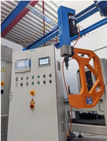
Example of a clinching pliers with NCFC servo press and BTM lightweight frame including clinching tool and maXYmos NC force-displacement monitoring system (Source: Kistler Group).
