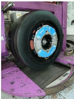
The wheel force transducer was validated on a tire testing machine at speeds of up to 250 km/h with the Kistler P530 multicomponent measuring hub.
