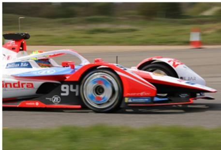
The RoaDyn Racing WFT accurately measures forces and moments acting on the wheels of racing cars to assess the tire's dynamic behavior.
