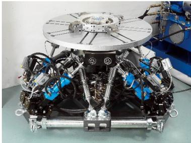
Several sensors of the type 9091B are built into the adjustable legs of this hexapod, which Kistler uses to calibrate other piezoelectric sensors.
