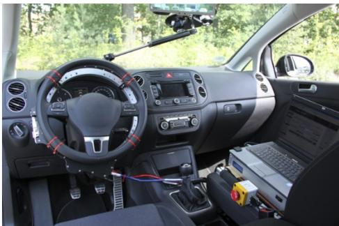
Torque sensors by Kistler combined with steering robots by Vehico measure driving dynamics and the functionality of ADAS systems.
