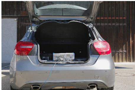
If the exhaust system vibrates too much, driving comfort is affected negatively. The 8248A3 miniature accelerometer provides reliable data in automotive vibration tests at up to 260 degrees Celsius.
