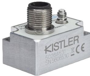
The new 5028A charge amplifier with IO-Link can output analog signals from piezoelectric sensors as digital measurement data, with the key advantages of flexibility, miniature format and lightweight design.
