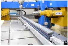
KiTraffic Digital enables the individual calibration of each quartz crystal, which significantly improves the accuracy of the sensor.
