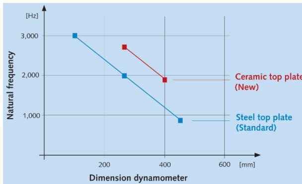
Dynamometers with a ceramic top plate offer significantly higher natural frequencies. Customers benefit because micro-vibrations with high-frequency content can be measured and reduced – leading to satellite images with vastly improved quality.
