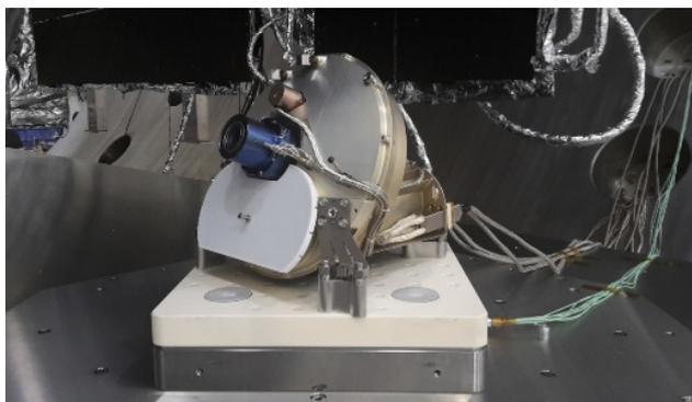
For larger satellite test units, Kistler offers the new ceramic-top piezoelectric dynamometer (9236A2) measuring 400 x 400 mm. (Source: Centre Spatial de Liège)
