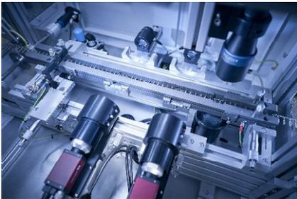
The KVC 621 punched part test cell measures and checks complex geometries and grid designs.
