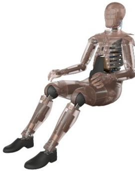
The THOR crash test dummy – a proprietary development – features sensors and DTI single-cable technology from Kistler, making it the leading complete system for crash tests.
