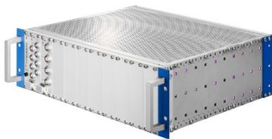
The KiDAU universal data acquisition system from Kistler was specifically developed for crash test dummy preparation and certification, and also for component tests.
