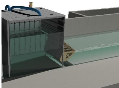
The tsunami researchers used sensors from Kistler that can measure forces in all three dimensions. Thanks to this technology, they were finally able to obtain precise measurements of the entire build-up of the wave in space and over time. (Source: © HR Wallingford [www.hrwallingford.com](http://www.hrwallingford.com))
