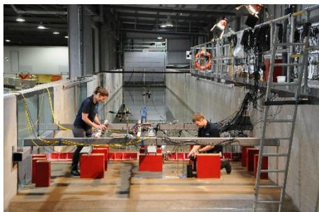
The English town of Wallingford is home to one of Europe's largest wave flumes, the Fast Flow Facility, where tsunamis can be simulated on a scale of 1:50. (Source: © HR Wallingford [www.hrwallingford.com](http://www.hrwallingford.com))
