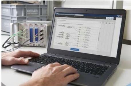
In combination with the KiStudio Lab software, KiXact makes the calculation and evaluation of measurement uncertainty simple and reliable.
