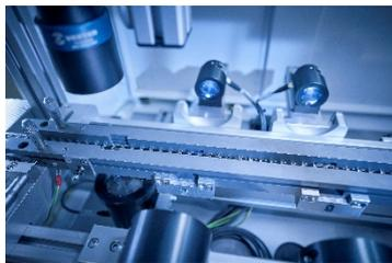
100% inspection with maximum efficiency: KVC 621 punched part test cell, configured here with 5 cameras
