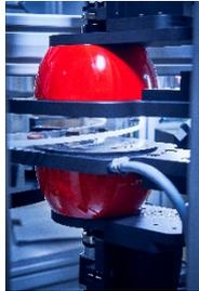
KVC 821: rotary plate and trevista® reflected light dome illumination unit, for challenging dimensional and surface tests on mass-produced parts
