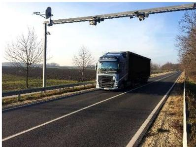
Weigh In Motion systems collect precise data about the loads exerted on roads and bridges.
