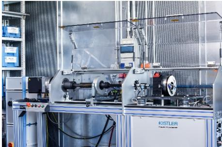
Kistler's Vibration Test System provides dynamic testing of the securing behavior of threaded joints
