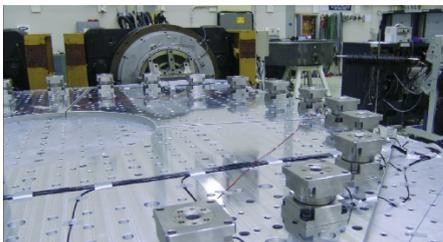
For Force Limited Vibration Testing, several preloaded 3-component force sensors are wedged between two metal plates. The structure is mounted on a shaker. The payload is positioned on the uppermost ring.
