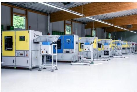
Quality assurance made easy: automatic testing and sorting systems from Vester – a Kistler Group Company – enable 100% control of plastic and hybrid parts.
