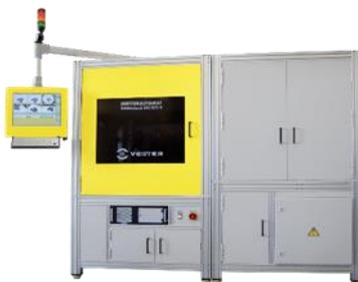
The VVC 821 automated testing system features a continuously rotating glass plate and allows correctly positioned camera inspection of up to 700 individual parts per minute.
