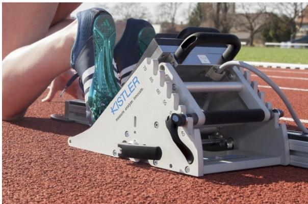
**Photo 3:** Equipped with sensors, Kistler's KiSprint starting block measures the force curve while a laser records the speed during the sprint start. (Source: Kistler Group)
