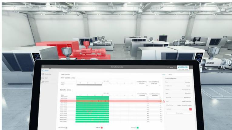
**Illustration 3:** ComoDataCenter is used to manage and analyze data for injection molding processes, and it allows networking of all ComoNeo and CoMo Injection systems.
