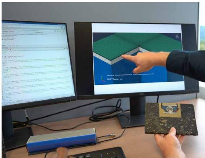
Data acquired from a Structural Road Analysis by Kistler is processed in simulations, leading to specific recommendations on the best sensor position and system layout for Weigh In Motion installations.
