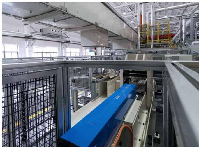
Kistler specifically designed this customized NCFN electromechanical joining system – with a very long stroke of 1,000 mm – for Yuchai, the engine manufacturer based at Yulin (China).
