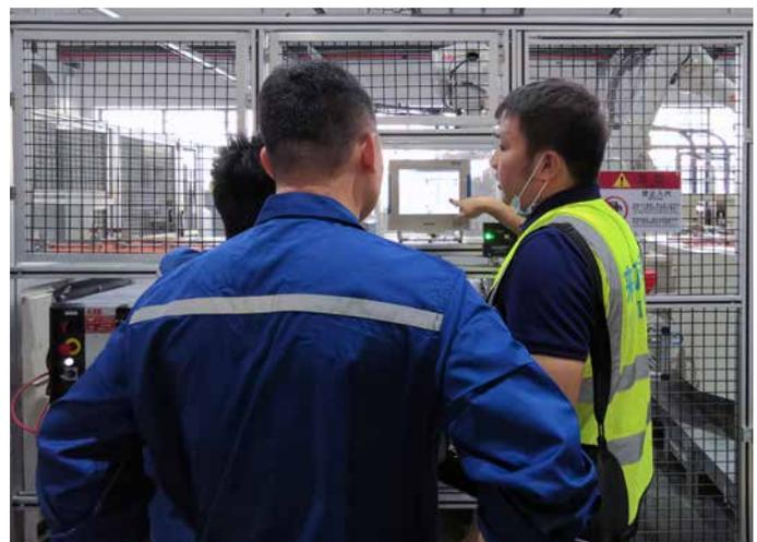
Production engineer Liu of Yuchai shows his colleagues how to handle the maXYmos NC process monitoring system for electromechanical joining systems from Kistler.
