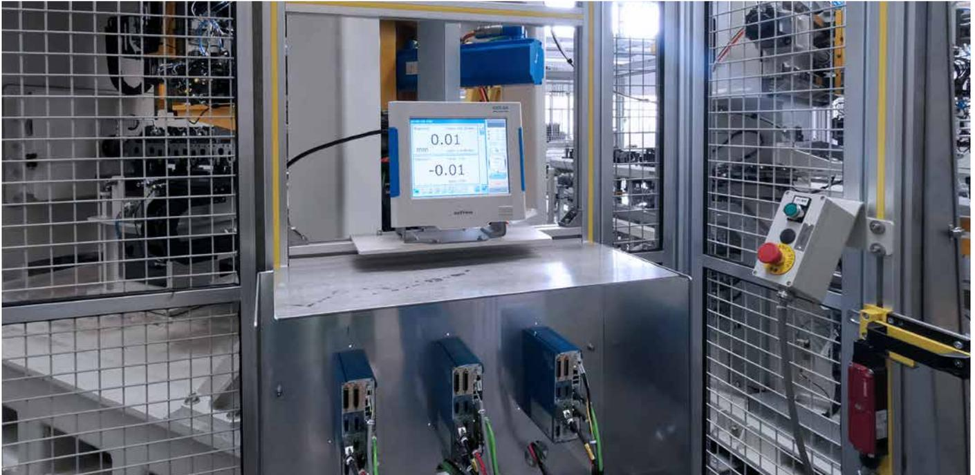
Three maXYmos NC process monitoring systems – with the matching display module – are used to control joining systems from Kistler at Yuchai's engine production plant in southern China.
