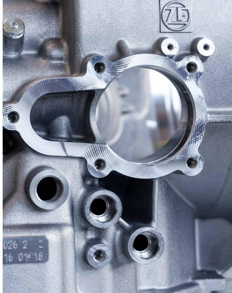
A component with different threaded joints
