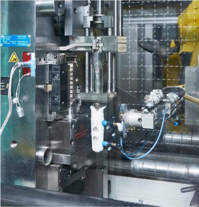
Sensor technology installed in the mold supplies the basis for transparent process management of all material-related and part-specific attributes – the part's 'fingerprint'
