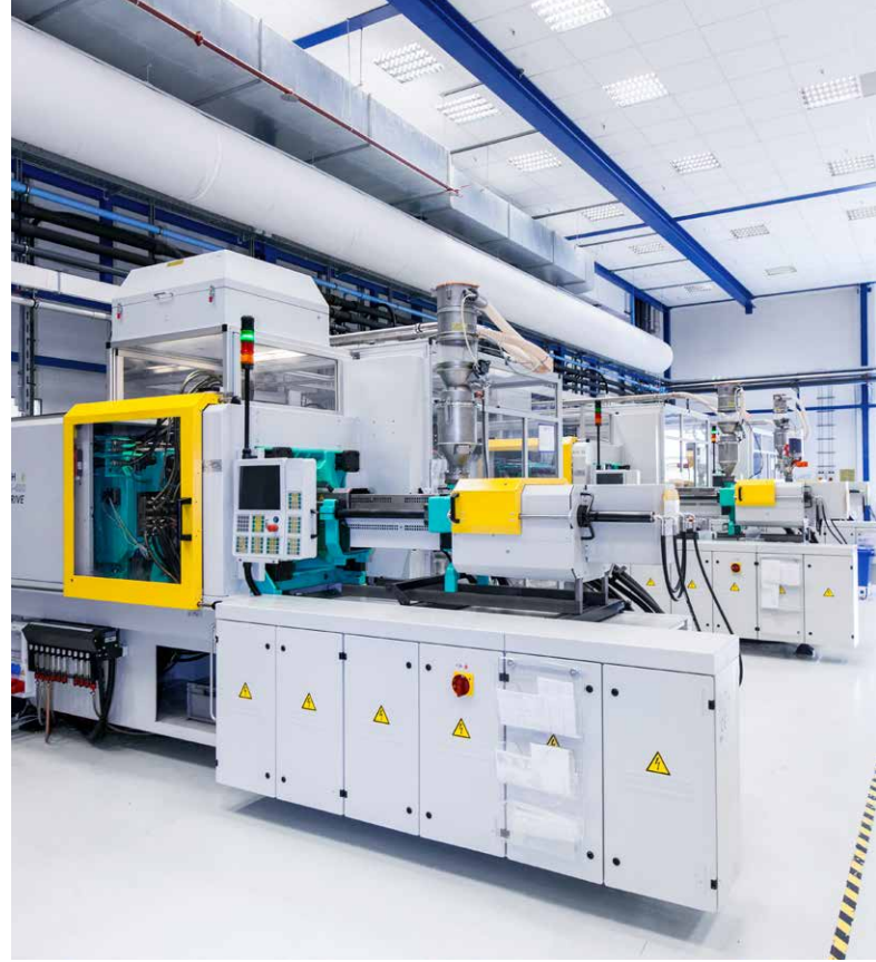
Cutting-edge injection molding plants operate with molds that have up to 96 cavities – and they are equipped with Kistler's ComoNeo process monitoring system
