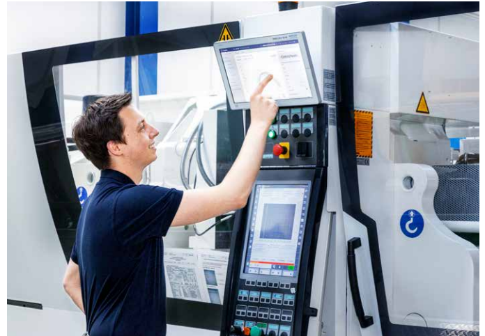
Cavity pressure monitoring with ComoNeo by Kistler makes easy work of process monitoring and quality assurance for injection molding
