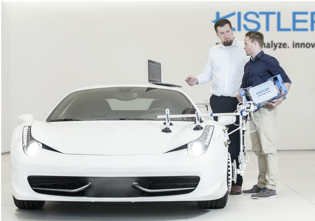
Precise measurements are an absolute necessity in combustion engine development. Kistler's KiBox Measurement and Evaluation System allows users to carry out complete combustion analysis in the vehicle and on the engine test bench. (Source: Kistler Group)
