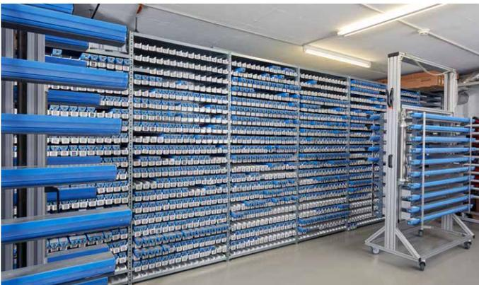
6 The finished sensors are placed in temporary storage before they are shipped to destinations across the globe, where they provide the centerpiece for Weigh In Motion systems from Kistler. Stocks of these sensors are continuously replenished to ensure rapid availability, even for large-scale projects.
