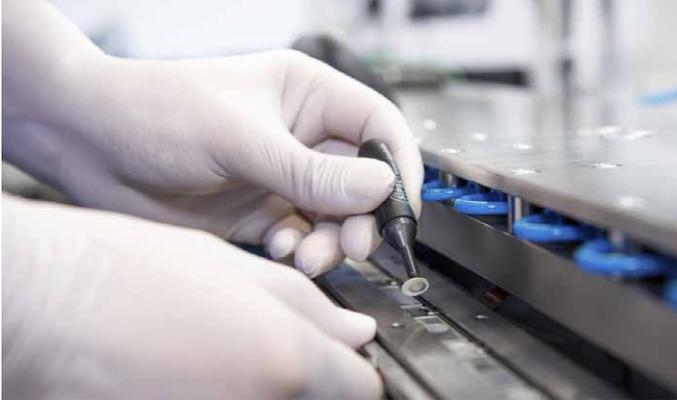
4 Once the quartz crystals are installed, final assembly of the sensor can take place. This includes installing the cables and sealing the sensor to make it airtight and waterproof. Finally, the aluminum profile is enclosed in a foam casing that dampens lateral forces.
