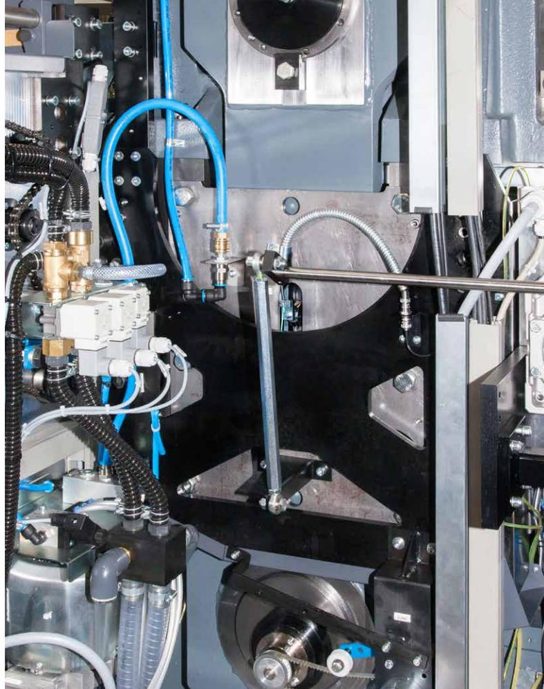
To prevent a blockade of the heavy machine, strain sensors by Kistler monitor the executed force during the entire process
