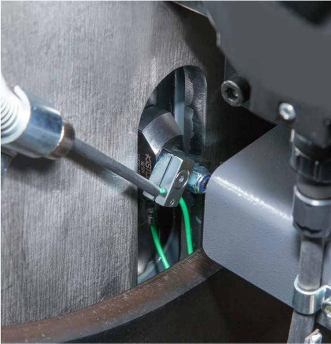
The strain sensors from Kistler are very robust and can be easily mounted or back fitted
