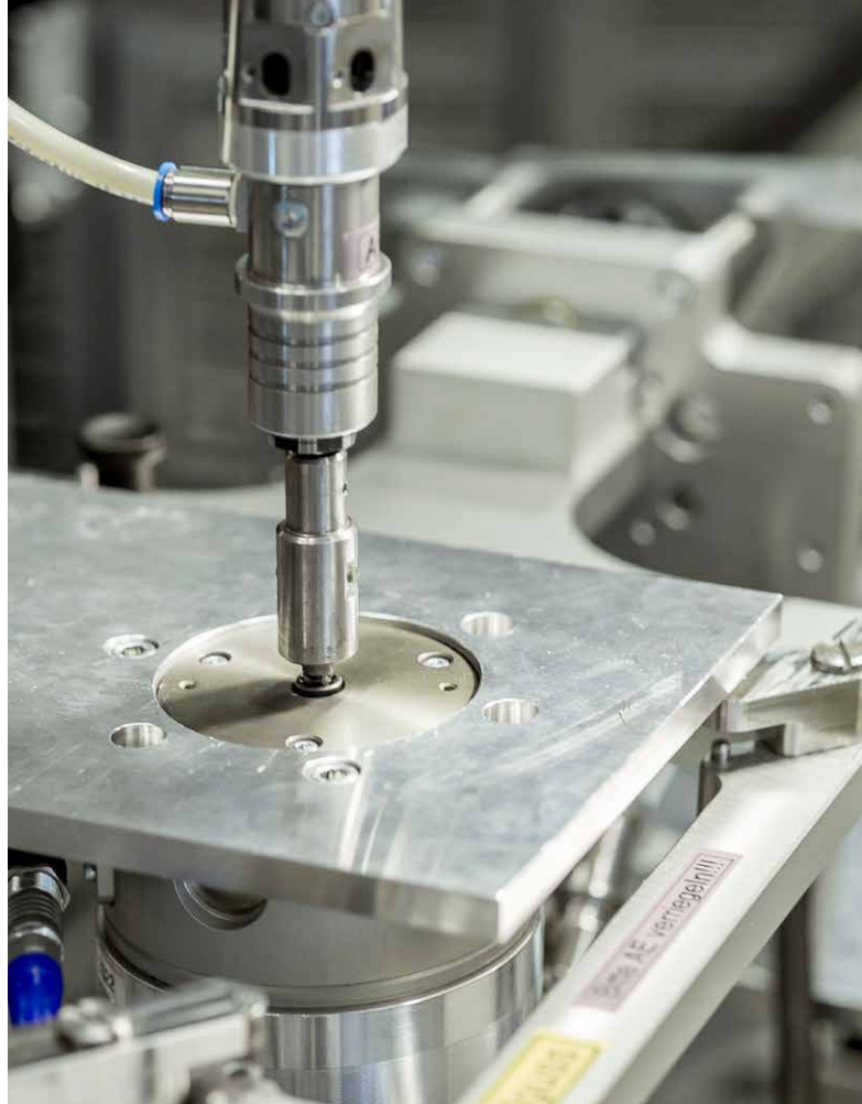
Since 2016, Zollner used combiTEST for standard-compliant testing and calibration of all torque tools, regardless of the manufacturer. The testing system from Schatz has been complemented by external simulators to avoid the need to dismantle tools for calibration purposes.
