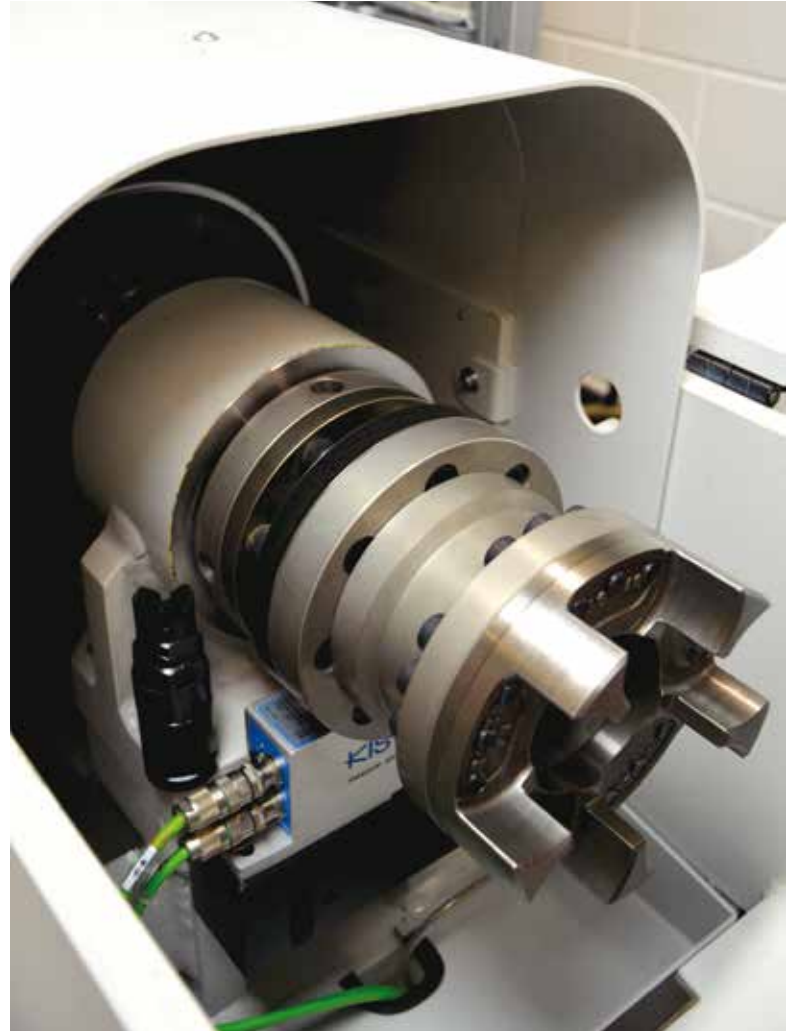
Kistler KiTorq Type 4550A, installed in the test rig
