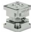
Types 9317C ... 9377C 3 axis force links Fx, Fy: \pm 1.5 \text{ kN} \dots \pm 75 \text{ kN} Fz: \pm 3 \text{ kN} \dots \pm 150 \text{ kN}
