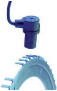
Fig. 10: Processing of the engine's stock crankshaft position sensor
