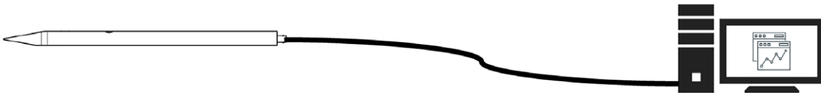
Fig. 2: Typical measuring chain for pencil probe Type 6233B...
