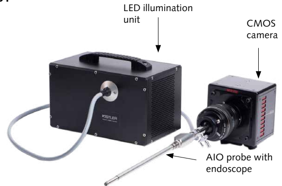
Fig. 2. Components of high speed camera imaging system
