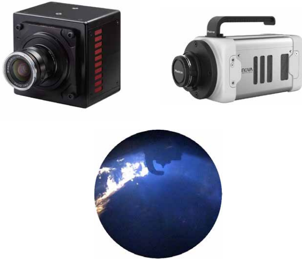
Fig. 4. High-speed cameras and sooting combustion of GDI engine
