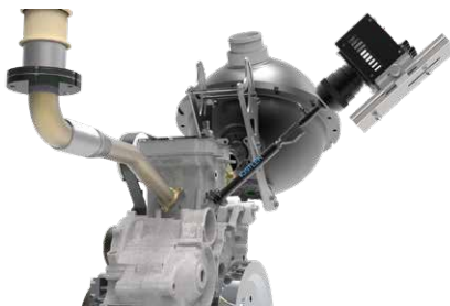
Fig. 1. Basic layout of high speed camera imaging system applied to single cylinder
