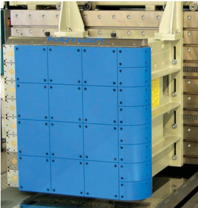
Fig. 5: Standard SmartCrash® segment, prepared for RCAR with profiled aluminium corner elements r=150 mm and aluminium front protection plates 250x250 mm
