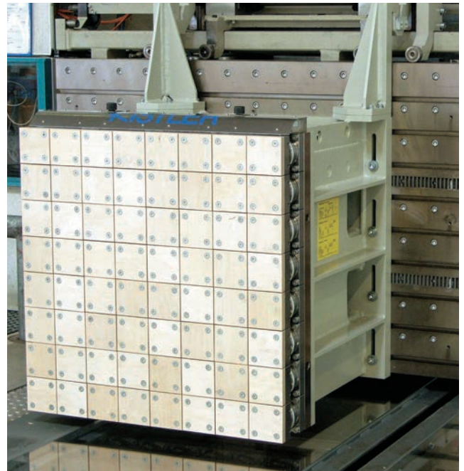
Fig. 4: Standard SmartCrash® segment, prepared for EuroNCAP with plywood protection plates, without deformable element (honey-comb)
