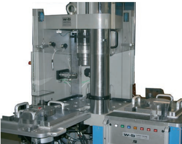
Fig. 10: Standard SmartCrash® force measuring element 125x125 mm
