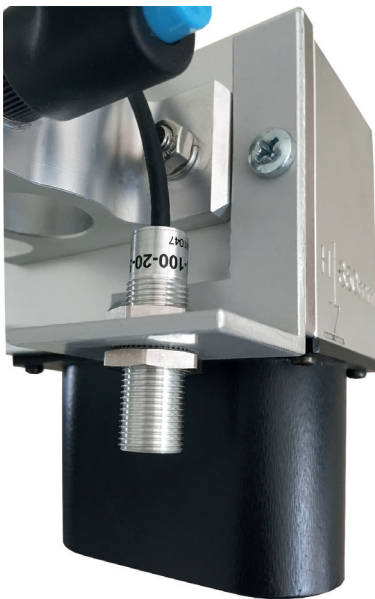
Fig. 2: IR Temperature Sensor Asphalt, mounted on a Correvit S-350 Sensor
