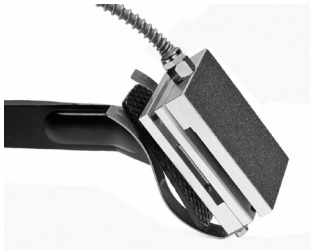
Fig 1: Sensor Type CPFTB mounted at the brake pedal
