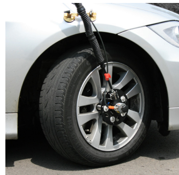
Fig. 2: WPT sensor mounted at the front wheel
