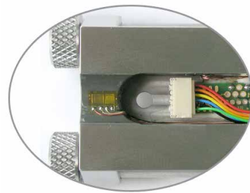
Fig. 3: Miniature connector inside load cell body
