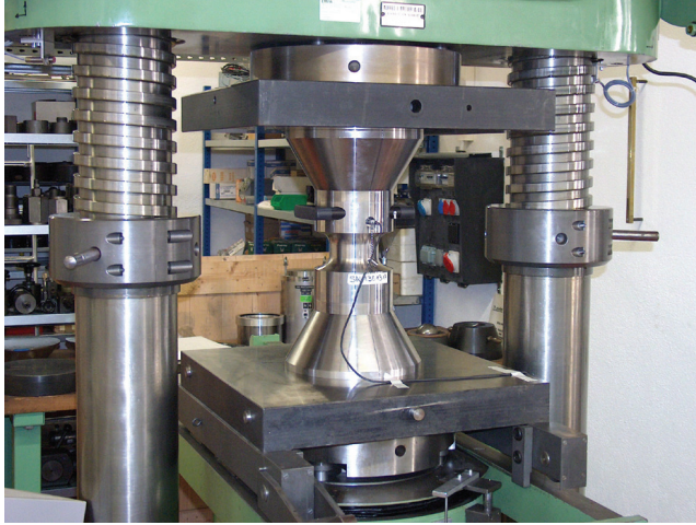
Fig. 8: Type 9931A2 (5 000 kN) meganewton press force calibration sensor
