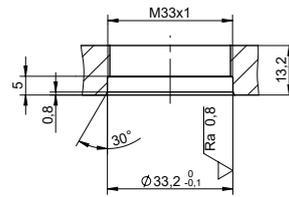
Fig. 5: Bore for thread mounting
