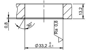
Fig. 6: Bore for flange mounting
