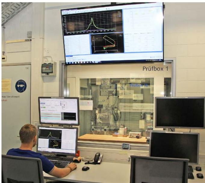
Image caption 2: Fast and efficient measurement with combustion pressure sensors at state-of-the-art Kistler engine test bench.
