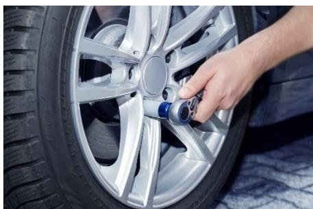
If you change your car tires yourself, you will experience how much force is needed: for a wheel bolt on a passenger car, you need to apply 100 to 110 Newton meters. But for the gigantic fasteners on a crane, the force required is sometimes about fifty times greater – and this can only be applied with the help of special tools.
