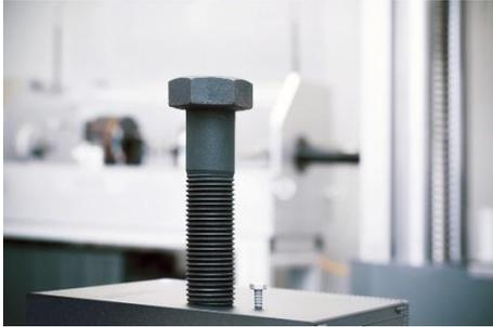
Test systems are already in operation for quality assurance of fasteners up to size M72, such as those used in wind turbines.
