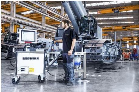
At Liebherr, the crane manufacturer, a technician uses a mobile test stand from Kistler to carry out daily checks that ensure the perfect functioning of a special tool used to tighten the gigantic fasteners on the crane. No crane leaves Liebherr's production line until its threaded joints have been perfectly tested – with inspection systems from Kistler.
