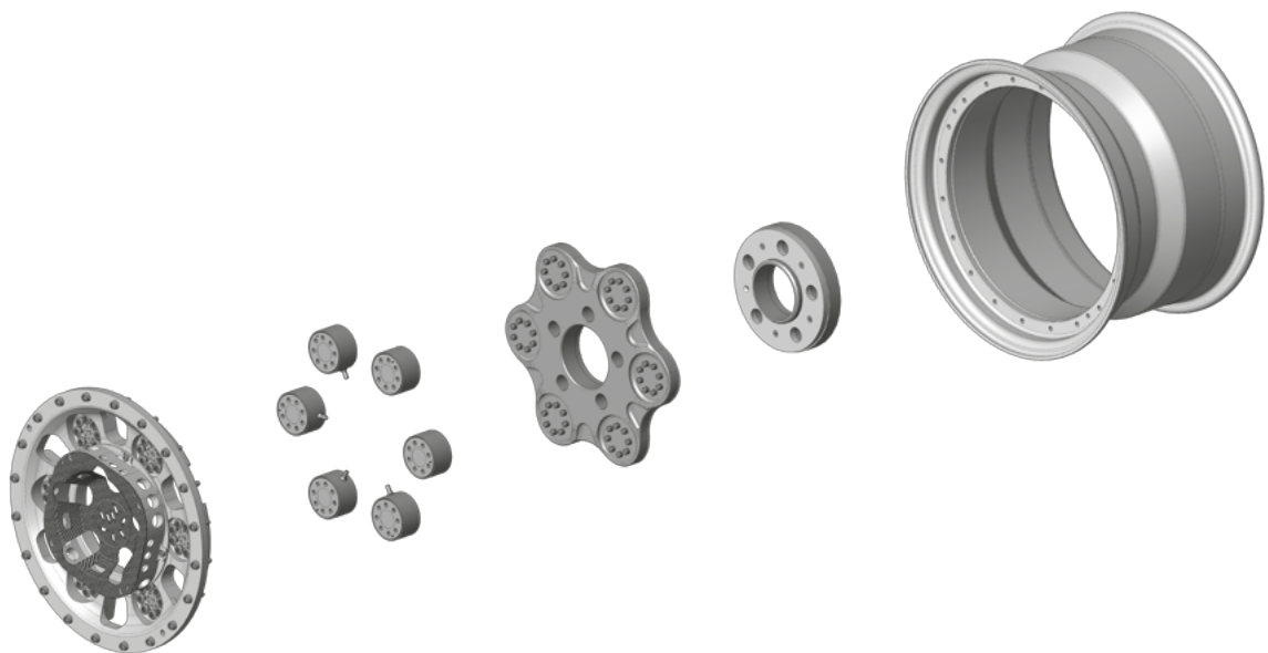
Fig. 2: RoaDyn® S660 structure/components for racing applications
