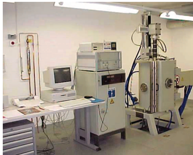
Crystal growing system according to the Czochralsky process (photo by Kistler)
