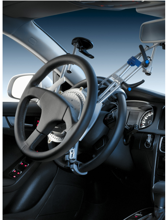
Fig. 9: Mounted Kistler MSW sensor with steering angle stop, steering wheel adapter, and stator mount
