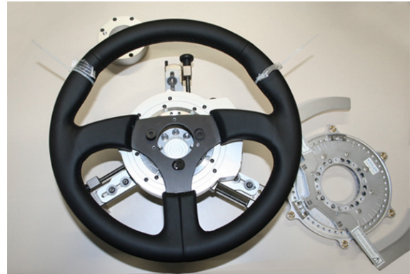
Fig. 1: Kistler MSW sensor with steering wheel, steering angle stop on the right
