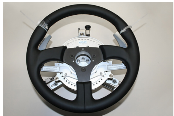
Fig. 6: Mounted steering angle stop
