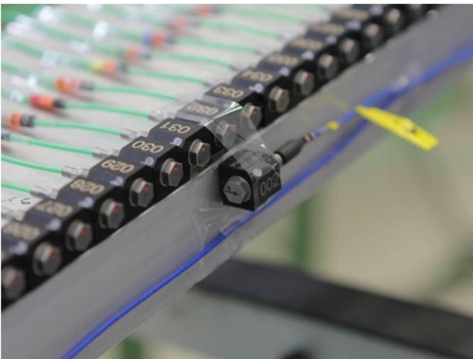
Fig. 9: Sensor installation of uni-axial application
