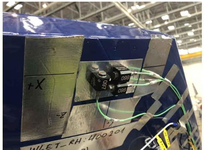
Fig. 10: Sensor installation of tri-axial application
