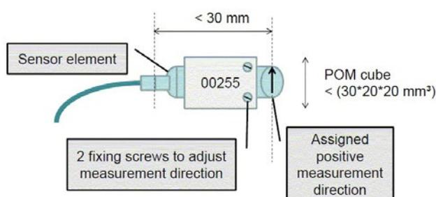
Fig. 4: Sensor and adapter requirements for adjusting sensitive direction
