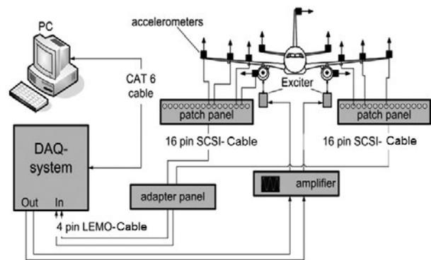
Fig. 1: Scheme of data acquisition for ground vibration testing at DLR
