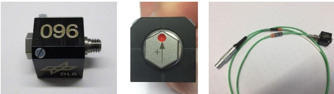
Fig. 8: Sensor Type 8000M095 with adapter 800M166 and cable assembly
