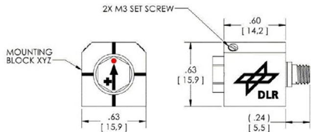
Fig. 7: Design of the insulating adapter Type 800M166 accommodating the sensor element Type 8000M095
