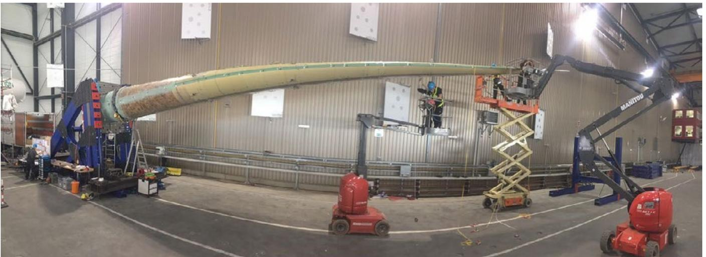
Fig. 11: Setup of measurement campaign on wind turbine blade
