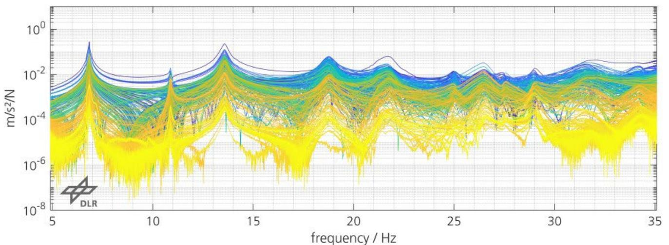
Fig. 14: Frequency response functions from time data of Fig. 13
