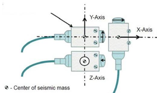
Fig. 5: Instance for triaxial planar arrangement of the accelerometer with COG marked
