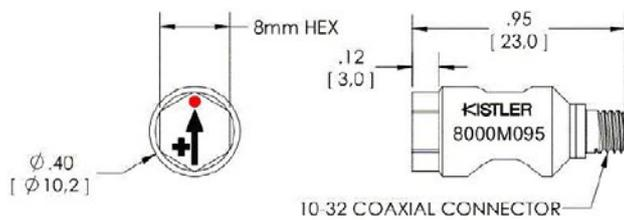
Fig. 6: Design of the sensor Type 8000M095
