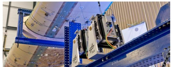
Fig. 3: Wind turbine blade modal testing performed by the German Aerospace Center from Göttingen Germany in February 2018
