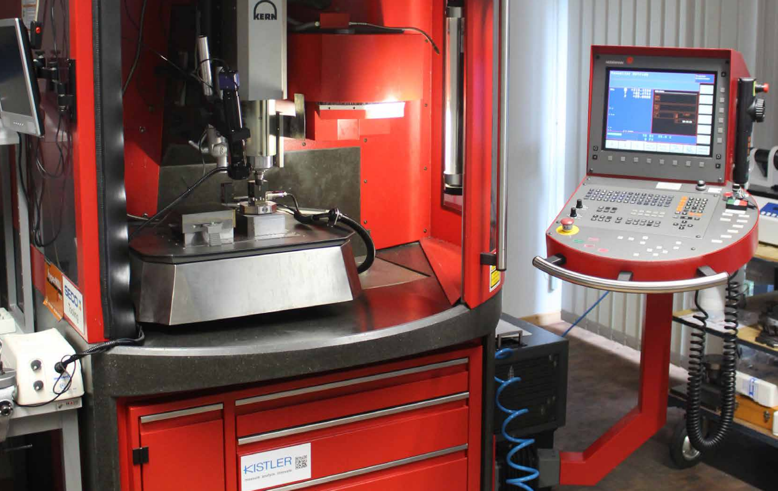
Research into machining using micro tools is conducted at the KERN HSPC 2522 micromachining center
