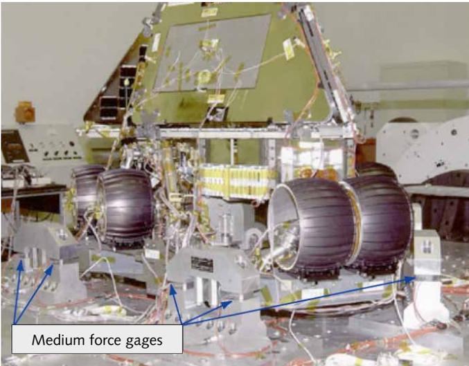
Fig. 6: The Mars exploration Rover "Opportunity" during an FLVT test. Eight 3-component force sensors (Type 9067C) were used
