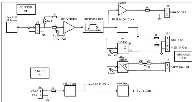
Fig. 4.: AE measuring chain block diagram
