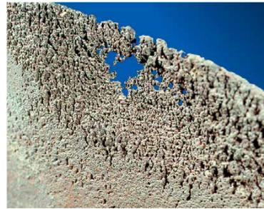
Fig. 7.: Example of cavitation damage. Source : Voith
