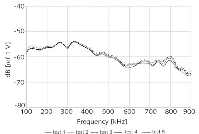
Fig. 2.: Repeatability of measurements tested and remounted using ¼-20 UNF 2A SHCS
