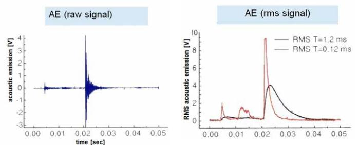
Fig. 5.: Raw AE signal vs RMS AE signal with signal averaging over 1.2 ms and 0.12 ms.
