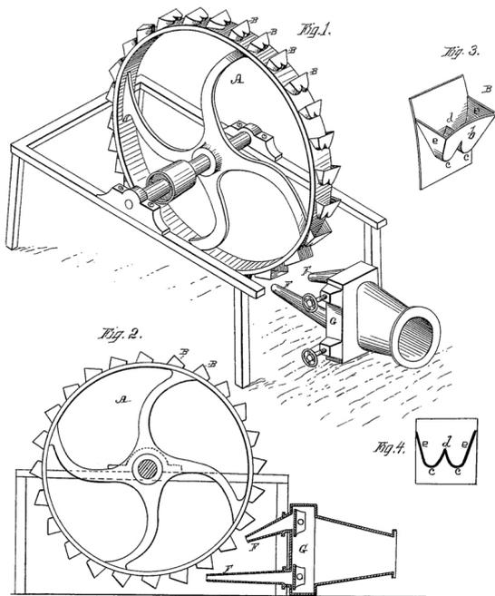
Fig. 6.: Figure from Pelton's original patent (October 1880) Source : L. A. Pelton - US patent 233692, page 1
